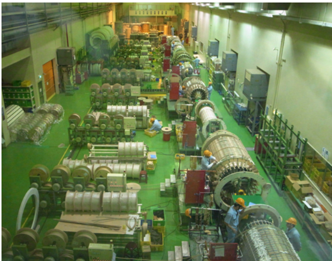
Winding Hall - Temperature and humidity controlled, dust-free clean room environment
